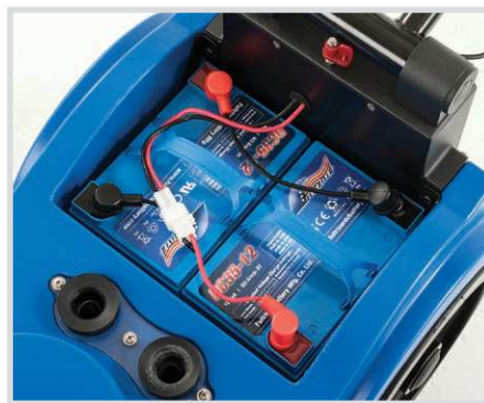
Maintenance-free AGM batteries and onboard charger.
