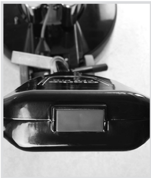
Safety lock-out switch.
